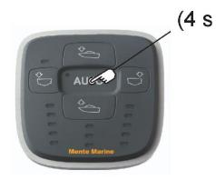
Run the boat at cruising speed. Manually control the trim tabs until you find the best attitude. Then, press and hold the auto button for 4 s, until the AUTO indicator is lit up.
