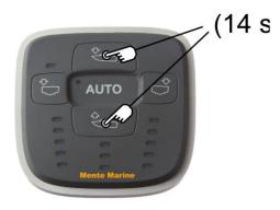
The AUTO indicator blinks to indicate that calibration is needed. Press the uppermost and lowermost buttons simultaneously for 5 s to start the calibration. Keep the buttons depressed for another 9 s, while the ACS is calibrating.
