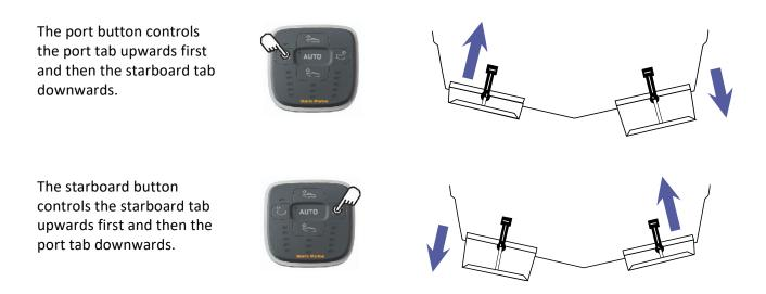
Should the trim tabs move in the wrong direction: For hydraulic trim tabs, exchange the 3 and 4 wires, for electromechanical trim tabs, exchange the 3 and 5 wires with the 4 and 6 wires.
