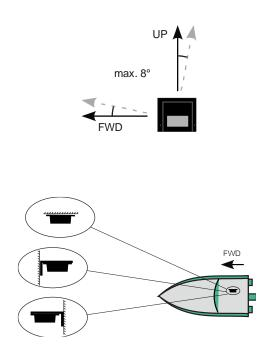
The control unit should be mounted in an upright position. The label on the front side is marked with an UP arrow that should point upwards and a FWD arrow that should point in the forward direction. Exact mounting is not critical, however, as the desired running attitude is set after installation.
