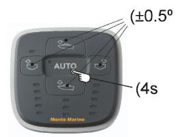
In the automatic mode, press any of the four buttons to alter the setting 0.5 degrees in a certain direction. Press more times for a greater change.
